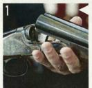
The process starts with a chat with the customer to discuss any noticeable problems, such as poor ejection. Next, the gun is checked for any cracks in the woodwork or knocks to the barrels. Gareth then looks at the functioning of snap caps and trigger-pulls and checks that the safety catch is working properly.
