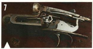
The bolt assembly is removed and cleaned. This Purdey is about 100 years old, but the internal parts don't seem to have aged. It is important that the bolt assembly is kept clean, to ensure that the gun opens and closes correctly
